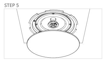
Attach the grill to the speaker by inserting the lips into the provided openings on the speaker baffle and rotating it over a partial turn (15°).
